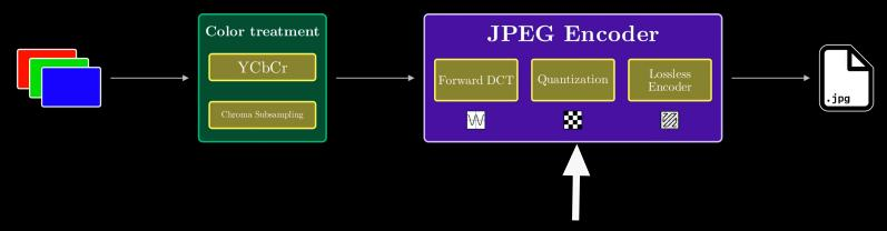
Different quantization tables For different compression rate
