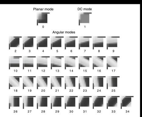
Fig. 4.2 Examples of  $8 \times 8$  luma prediction blocks generated with all the HEVC intra prediction modes. Effects of the prediction post-processing can be seen on the top and left borders of the DC prediction (mode 1), top border of horizontal mode 10 and left border of vertical mode 26
