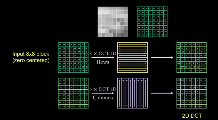
STEP-2: 2D DCT of each 8x8 block
