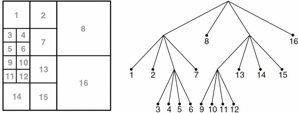
**Fig. 3.4** Example for the partitioning of a  $64 \times 64$  coding tree unit (CTU) into coding units (CUs) of  $8 \times 8$  to  $32 \times 32$  luma samples. The partitioning can be described by a quadtree, also referred to as coding tree, which is shown on the *right*. The numbers indicate the coding order of the CUs
