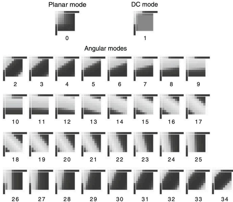
**Fig. 4.2** Examples of  $8 \times 8$  luma prediction blocks generated with all the HEVC intra prediction modes. Effects of the prediction post-processing can be seen on the top and left borders of the DC prediction (mode 1), top border of horizontal mode 10 and left border of vertical mode 26
